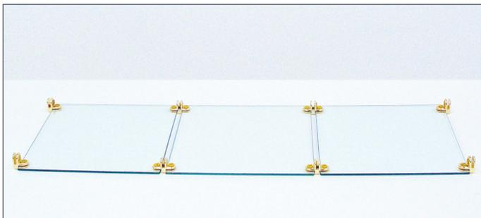
**Step 1:** Arrange the glass lites on the base surface which represent the number of cubes wide. Clean the bottom surface of the glass. As illustrated, attach 2-Way Connectors on the end lites and 3-Way Connectors between the lites. Use a wide blade screwdriver for Z-Line Connectors or a soft face rubber mallet for Clear Plastic Connectors.
