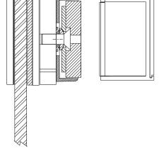
Place standard template on HDB bracket with the armature hole drill position (on template) over the armature hole in the HDB bracket. Tape the template in place. Mark and drill required holes in frame. Follow installation instructions for the model being installed.
