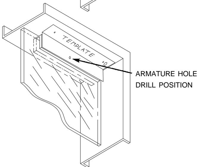
Place standard template on HDB bracket with the armature hole drill position (on template) over the armature hole in the HDB bracket. Tape the template in place. Mark and drill required holes in frame. Follow installation instructions for the model being installed.
