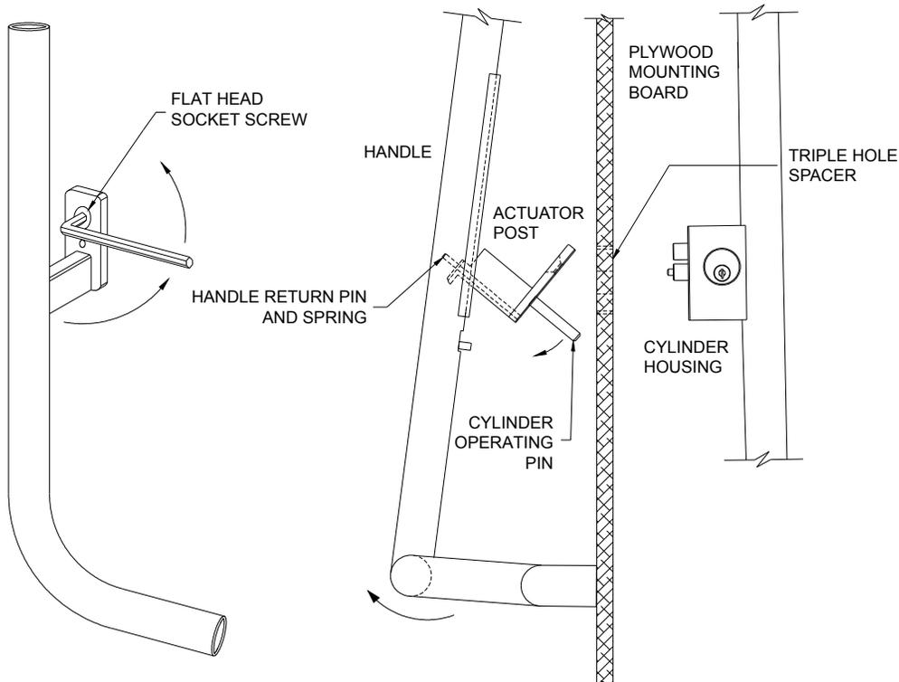
2. FOR RAIL MOUNT HANDLE. Rotate round connector pivot fitting counter clockwise and remove from Adapter Block. Note: Use pliers and rubber strip (to protect finish) for removal of round connector. ➔
