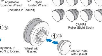
NOTE: Lower Rollers are installed after doors are hung. See Page 10.
