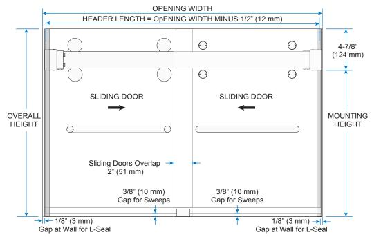
NOTE: Drawings not shown to scale. Header Bar is cut 1/2" (12 mm) less than Opening Width. Use wall-to-wall tight dimension. Overall Height is height from curb/floor to top of glass.
