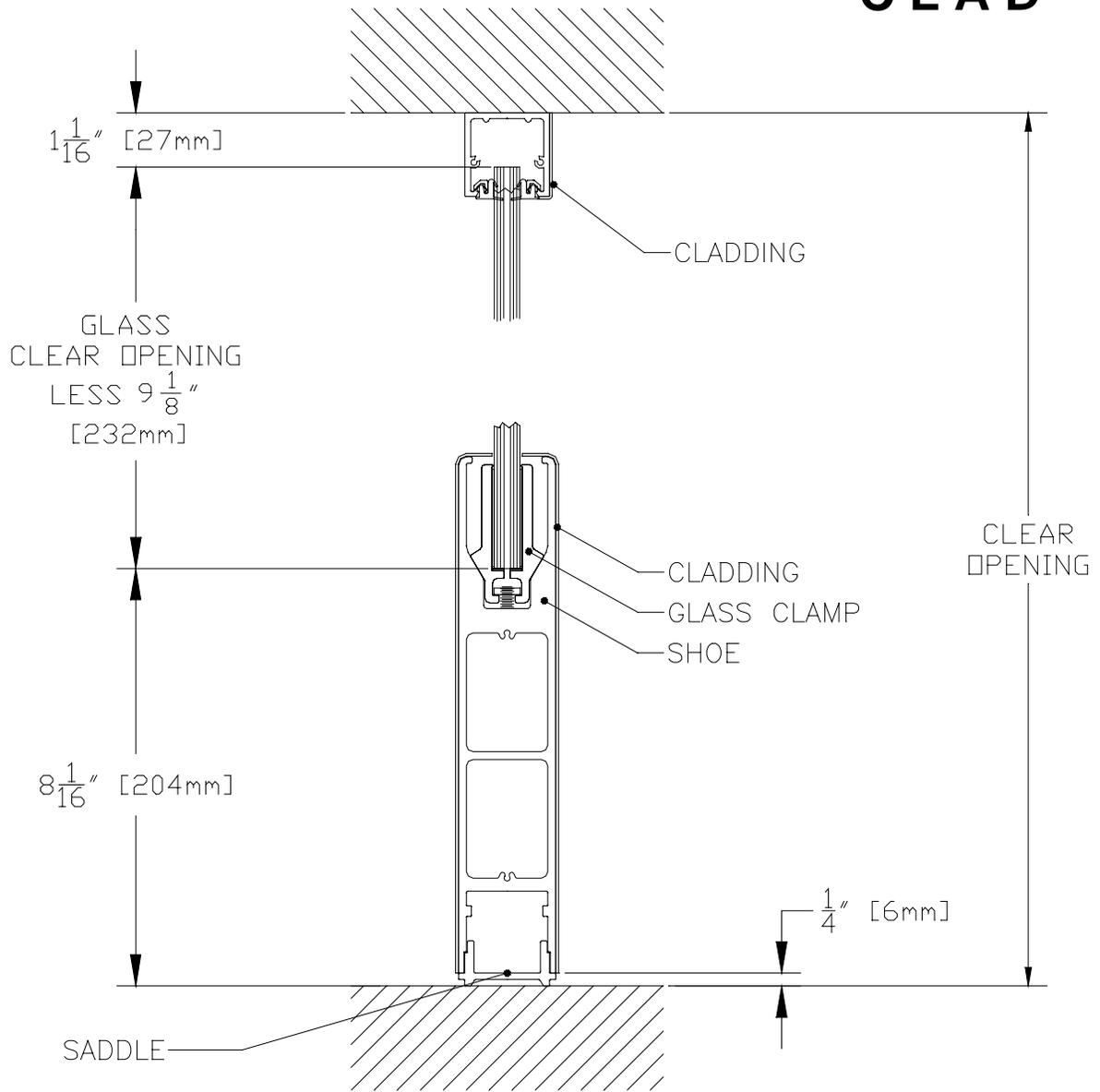
U-CHANNEL TOP CLAD OR NON CLAD
