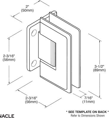
to Ensure Accuracy Wall Mount Hinge - Short Back Plate
