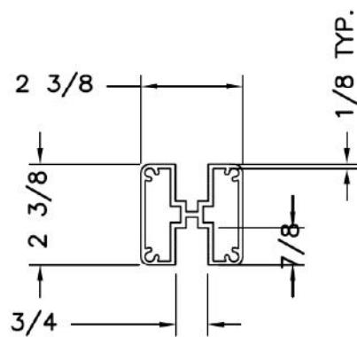
Design of the aluminum post is according to the 2015 Aluminum Design Manual. 6061-T6 aluminum is assumed in the calculations. Use ADM Design Table 2-19.
